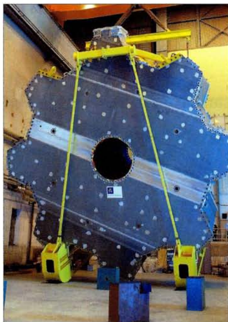
One of the 11 m high vacuum vessels for the two ATLAS endcap toroids – typical of the large pieces that will be lowered into the cavern during the installation process.
