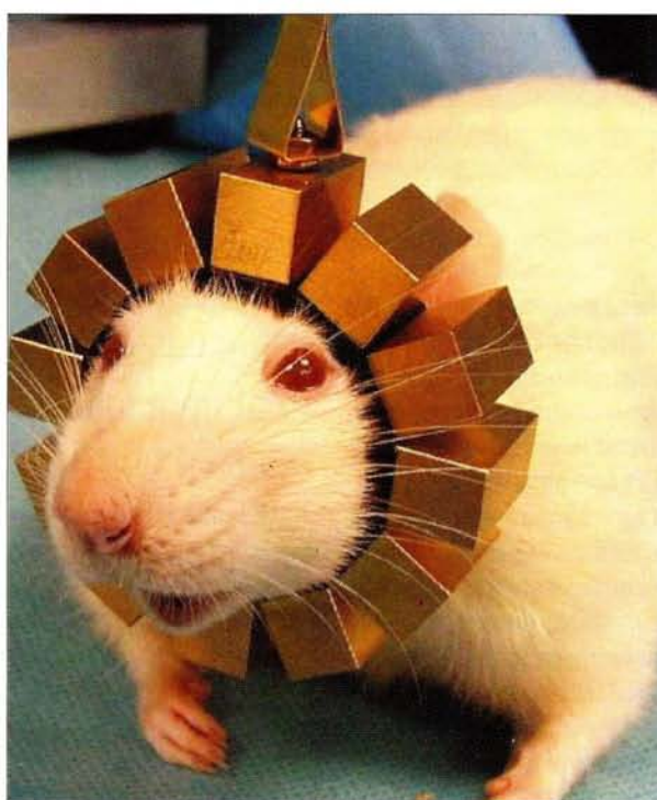
A small, head-mounted PET tomograph for imaging the brain of a rat while awake. (Courtesy of Craig Woody, BNL.)
