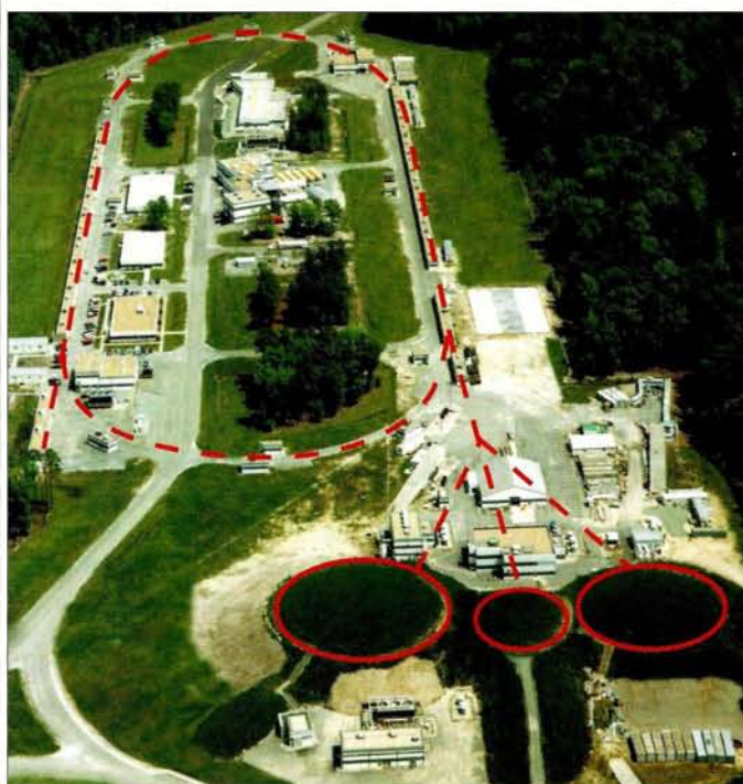
An aerial photograph of the Continuous Electron Beam Accelerator Facility (CEBAF) at Jefferson Lab. The dashed line indicates the location of the accelerator, and the circles indicate the location of the three experimental halls.
