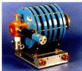
SUPERNANOGAN: An ECR source with permanent magnet for low and high charge state. (H + : 2mA, Ar n+ : 350µAe)
